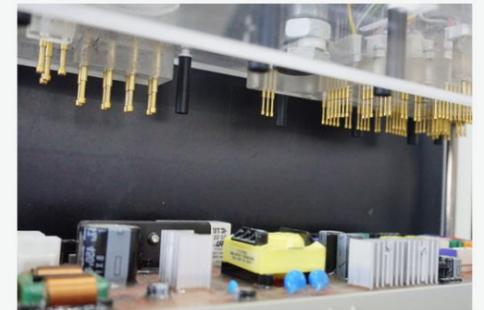
Heating component is the core part of smart toilet. iKAHE will execute the test of sensors, power consumption, water temperature and so on.
